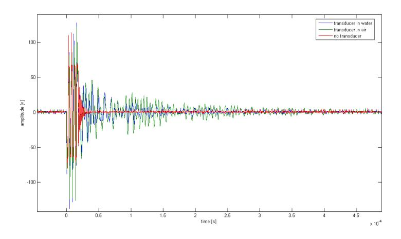
Waveforms of the of the piezo transducer ringdown (Airmar P319).
